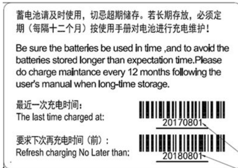
Figure 5-1 Battery charge label
